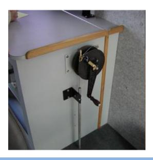
Optional pipe and pulley system, allows winch to be located above engine spaces or other obstructions mounted above sea chest.
